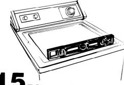
Tilt washer forward, raising back legs 1 inch (2.54 cm) off of floor to adjust rear self-leveling legs. Gently lower washer to floor. Check levelness of the washer by placing a carpenter's level on top of the washer, first side to side; then front to back.
